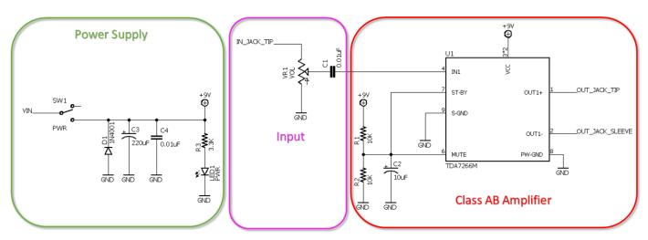
The design is based on a simple dual bridge, class AB amplifier.
